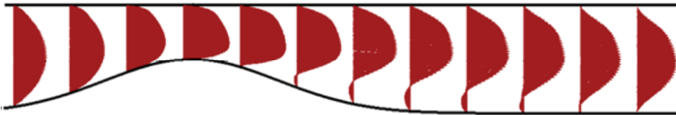
Fig. 5. Velocity profile, with an appreciable recirculation zone, in the asymmetric tissue culture model at 6.25 dynes/cm 2 .
