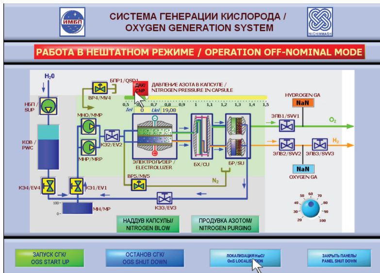
Fig. 12. Front panel of the 'OGS' virtual simulator subroutine in 'OPERATION OFF-NOMINAL MODE' (Pressure in the canister is below norm.).
